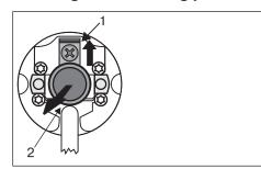
When pushed in, the mounting pin (2) locks automatically. To undo the mounting pin (2), push the tab washer (1) upwards and pull out the mounting pin (2).
