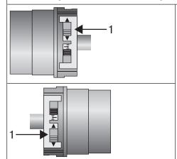
Switch the direction switch (1) to the opposite position.
