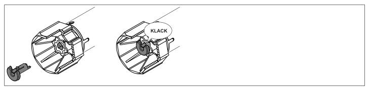
Assembling and disassembling the drive adapter with screw connection
