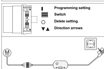
Connect the wires of the tubular drive to those of the same colour in the cord switch set or operator control and switch on the power supply.
