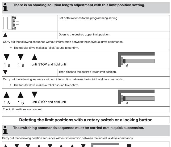
The tubular drive acknowledges. Both limit positions are deleted.
