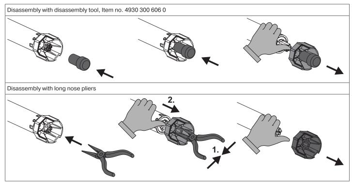
Assembling and disassembling the drive adapter with separate drive adapter safety catch
