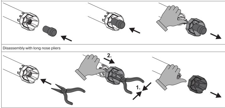
Assembling and disassembling the drive adapter with separate drive adapter safety catch
