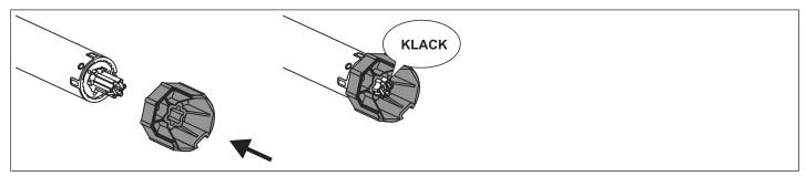
Disassembling the drive adapter with safety catch on the drive shaft
