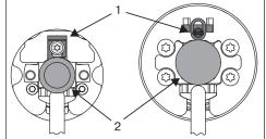
When pushed in, the mounting pin (2) locks automatically. To undo the mounting pin (2), push the tab washer (1) upwards and pull out the mounting pin (2).
