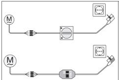
Automatic setting of limit positions is possible, where a stop system is present on both sides, using the switch (Item no. 4901 001 158 0), a standard rotary switch or the programming unit for drives with electronic limit switching (Item no. 4935 200 011 0). All other functions can only be set via the programming unit.
